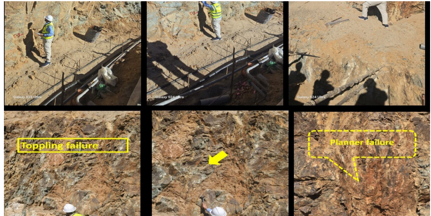
Field mapping of rock-face failure mechanisms
